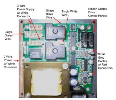
NOTE: You may or may not have the 2 wire power connector. It does not matter which ribbon cable goes on which conneter.
